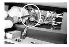
5) Disconnect the DC spark generator wires from the valve.
